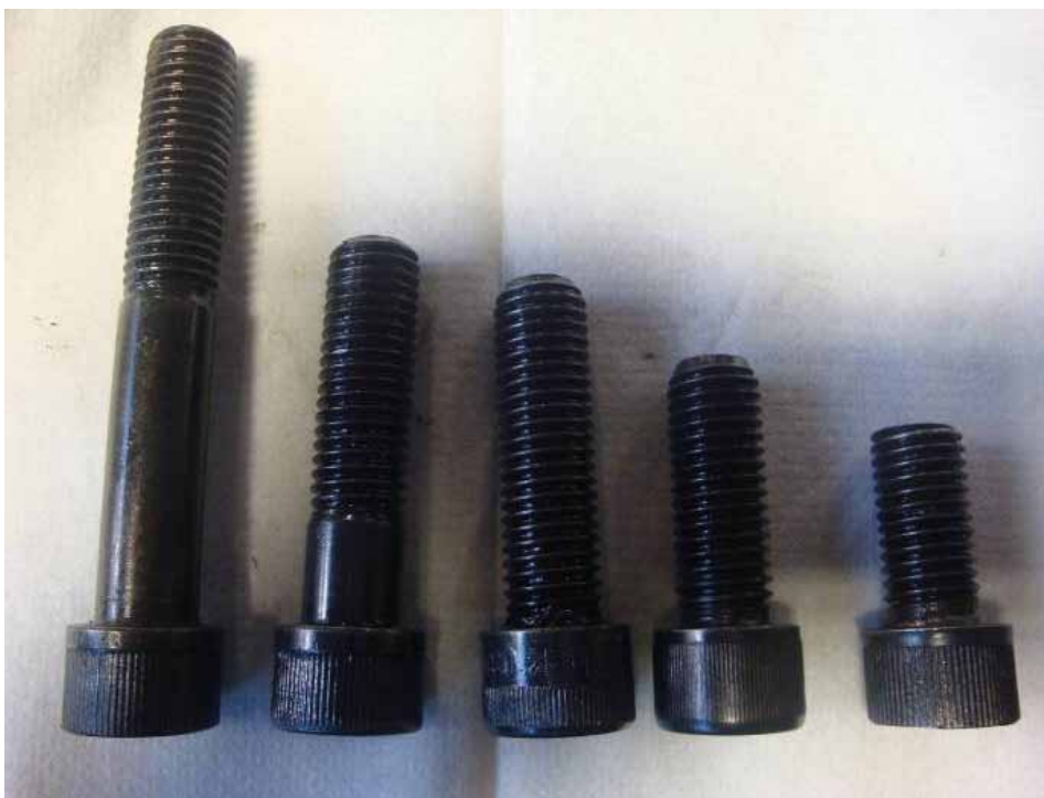
In the photo above, these five bolt lengths were used to change-over from one die set to another die set!
