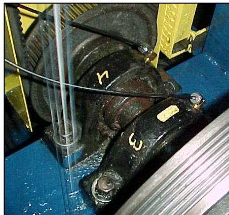
Weekly Operator Lubrication - 8 Lube Points for the Wire Draw machine
