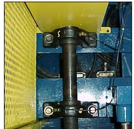
Weekly Operator Lubrication - 8 Lube Points for the Wire Draw machine
